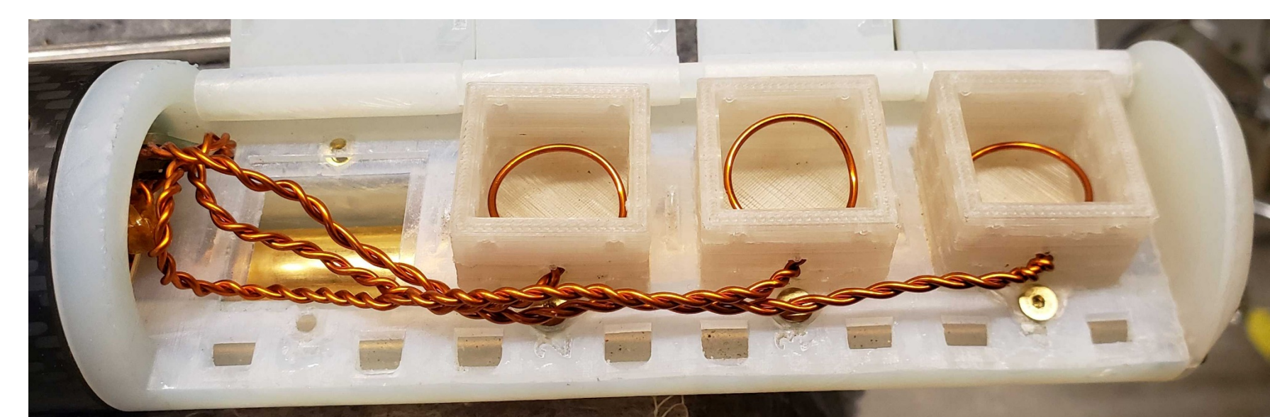
DNP target ladder with NMR coils and rectangular 3D-printed Kel-F cups after cooling to 1 K. The cup on the far left was removed to allow access to electronics.
